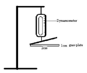
**Figure 1.** Device for the adhesion force measurment.
